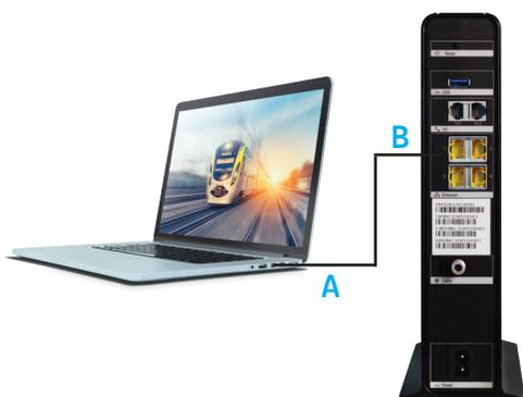
A. To create a hardwired connection to your device, connect one end of the Ethernet cable to your device's Ethernet port.
