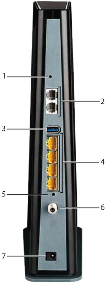
1. **Reset button:** resets the Telephony Gateway as if you power cycled the unit. Use a pointed non-metallic object to press this button.
